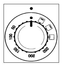
If you turn the secondary oven function selector and thermostat control knob anti-clockwise, it will automatically select the conventional oven function and you can regulate the temperature between 50 - 250°C.
