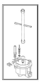
Unscrew the injector and replace it with the stipulated injector for the new gas supply (see table on next page).
