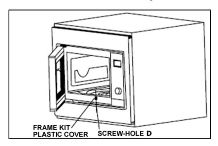
o Use the frame kit plastic cover and place it over screw-hole D.
