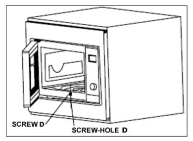
Open the microwave door and locate screw-hole D. Use screw D to fix the microwave oven to the housing unit.
