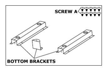
For the next step in the preparing the housing unit process, you will require 10 x screw A and the bottom brackets.
