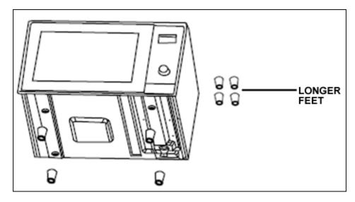
o Carefully turn over the oven and replace the existing feet, with the longer feet supplied in the installation kit.
