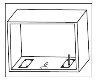
You should make marks on the base of the housing unit, in the positions marked with the letter "a" on the template.
