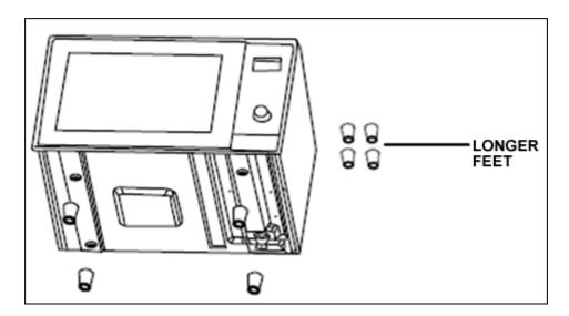
o Carefully turn over the oven and replace the existing feet, with the longer feet supplied in the installation kit.
