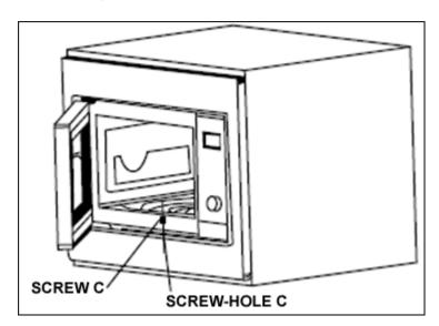
o Open the microwave door and locate screw-hole C. Use screw C to fix the microwave oven to the housing unit.
