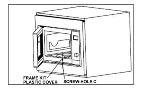
o Use the frame kit plastic cover and place it over screw-hole C.
