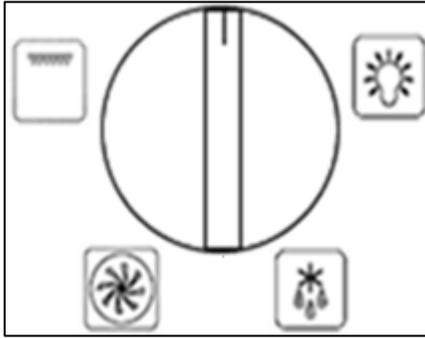
The main oven function selection knob should be used to select the particular mode of cooking that you require. The appliance will utilise different elements within the oven cavity, depending on the oven function that you select. When a function is selected, the main oven power indicator light will come on.
