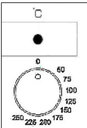
The oven thermostat control knob sets the required temperature of the oven. It is possible to regulate the temperature within a range of 50 - 250°C.
