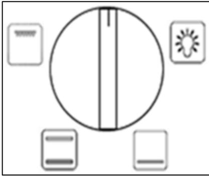
The secondary oven function selection knob should be used to select the particular mode of cooking that you require. The appliance will utilise different elements within the oven cavity, depending on the oven function that you select. When a function is selected, the secondary oven power indicator light will come on.
