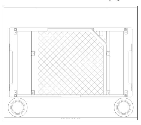
4) After fitting the carbon filter, the underneath of the cooker hood should appear as in the drawing opposite.
