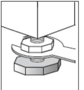
✓ Slacken off the lock nut on each of the washer dryer feet using a spanner.
