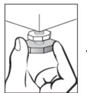
✓ Adjust the feet to level off the washer dryer.
