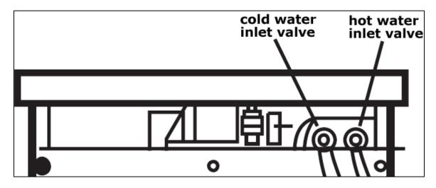
• When you are facing the **rear** of the appliance, you will see two water inlet valves next to each other. The cold water inlet valve is on the left hand side and the hot water inlet valve is on the right hand side.
