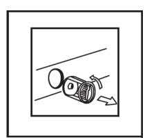
When all the water has drained out of the washer dryer, turn the filter several times anti clockwise, until it can be removed completely.
