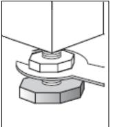
✓ Once levelled correctly, you should tighten the lock nut back up on each of the washer dryer feet using a spanner.
