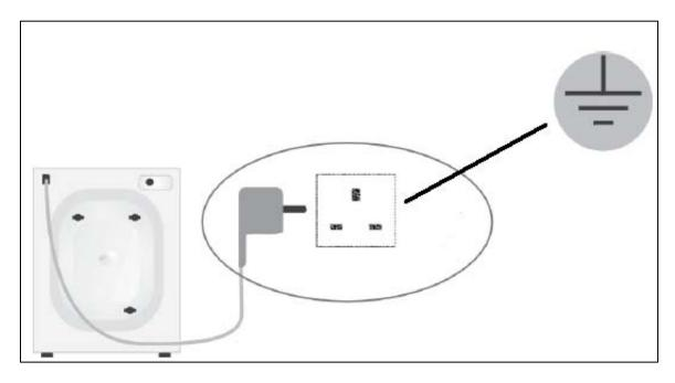
✓ IMPORTANT: The electrical socket must still be accessible once the appliance is installed.
