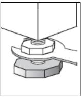
✓ Slacken off the lock nut on each of the feet using a spanner.
