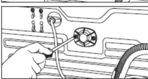
✓ Using a screwdriver, refit the three plastic transit bolt covers that you removed previously.
