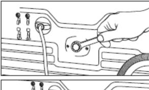
✓ Loosen and remove the three transit bolts.
