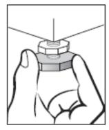
✓ Adjust the feet to level off the washer dryer.
