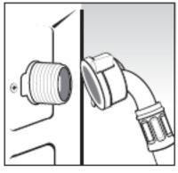
✓ Connect and fully tighten the inlet hose to the threaded inlet valve that is located at the rear of the washer dryer. You should connect the end with the right angle connector on it to the back of your appliance.
