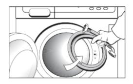
✓ The water inlet hose will be inside the drum of your washer dryer, when you receive the appliance.
