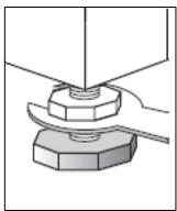
Once levelled correctly, you should tighten the lock nut back up on each of the feet using a spanner.
