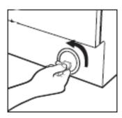
Remove the kickplate and then use a coin to turn the filter cap.
