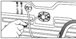
✓ Using a screwdriver, unscrew the three plastic transit bolt covers.
