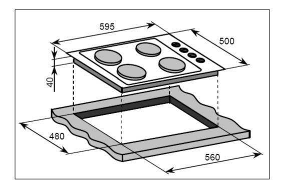
Cut a hole in the worktop that corresponds with the drawing shown above.
