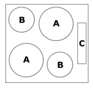
A = 1.50 kW thermostatic plate ( $\emptyset$  180 mm) B = 1.00 kW thermostatic plate ( $\emptyset$  145 mm)
