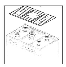
Remove the pan-stands, burners and flame spreaders.
