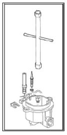
Unscrew the injector and replace it with the stipulated injector for the new gas supply (see table below).
