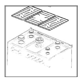
Remove the pan-stands, burners and flame spreaders.
