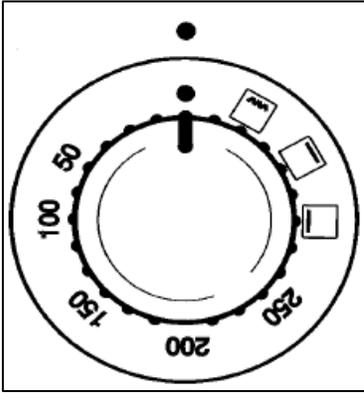
If you turn the secondary oven function selector and thermostat control knob anti-clockwise, it will automatically select the conventional oven function and you can regulate the temperature between 50 - 250°C.
