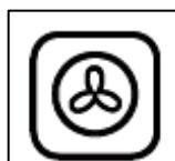
**FAN OVEN:** This method of cooking uses the circular element while the heat is distributed by the fan. This results in a faster and more economical cooking process. The fan oven allows food to be cooked simultaneously on different shelves, preventing the transmission of smells and tastes from one dish onto another.
