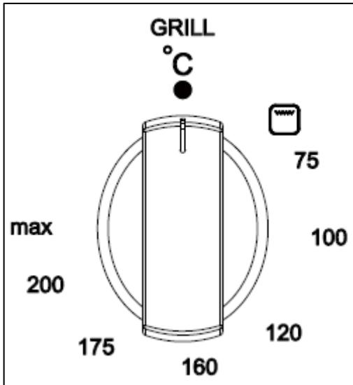
The grill control should be turned clockwise and used to select the grill temperature that you require. We recommend that you preheat the grill for five minutes before putting food into the grill.
