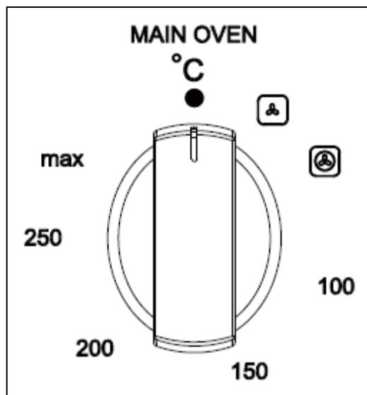
The oven temperature control should be turned clockwise and used to select the particular mode of cooking that you require. If you turn the dial clockwise and select the first symbol, this will start the defrost function. If you continue turning the dial and set the oven to a temperature, then the fan oven setting is selected.
