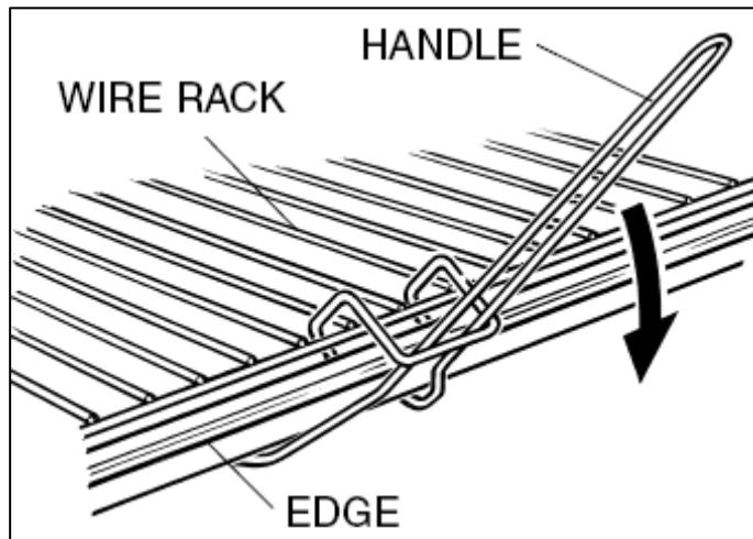
**IMPORTANT:** When fitting the handle to the enamelled baking tray, hook the handle over the edge of the tray and through the wire rack at a central point, along the tray edge. Lower the handle fully down to secure it.
