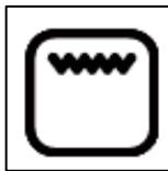
**FULL GRILL:** This method of cooking utilises the inner and outer parts of the top element, which directs heat downwards onto the food. This function is suitable for grilling medium or large portions of sausages, bacon, steaks, fish etc. Ideally the thermostat control knob should be set to 200°C
