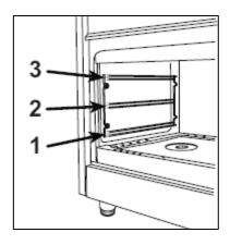
The oven walls are fitted with various guide bars on which you can place an oven shelf or a drip tray (see image below).
