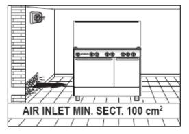
These apertures must be positioned in such a way as not to be obstructed.
