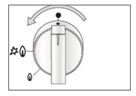
Press the relevant burner dial and rotate anticlockwise to the large flame icon. Release the dial and the burner will automatically ignite. Matches can also be used to light the burner during a power cut.
