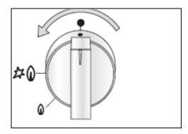
Turn the relevant dial anticlockwise to select a power level for a chosen burner.
