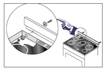
Fix the back-guard into place by screwing the screws back into the hob with the back-guard placed in between.
