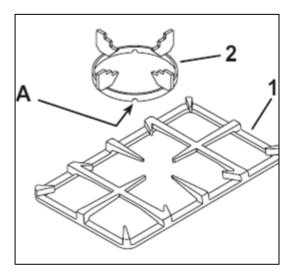
The appliance is equipped with pan supports (1), on which the wok support (2) must be placed. To ensure stability, position the notch (A) of the wok support on the pan support fingers as indicated in the diagram above.
