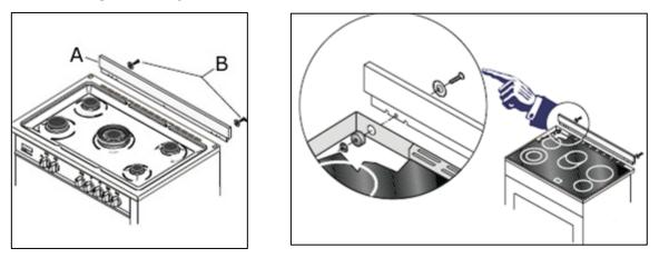
• Fix the back-guard into place by screwing the screws back into the hob with the back-guard placed in between.
