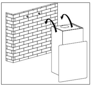
**5)** Screw the anchoring screws through the relevant holes in the cooker hood. Fully tighten the anchoring screws into the wall.
