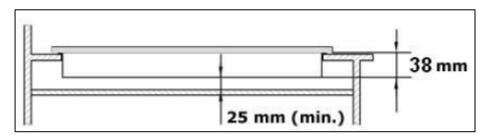
• **IMPORTANT:** You must have a gap of at least 25 mm between the underneath of the appliance and any surface that is below it.
