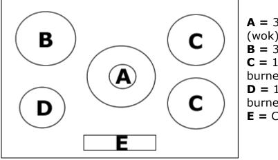
A = 3.80 kW triple crown (wok) burner
