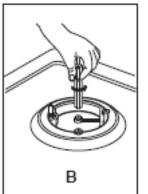
Unscrew the injector (B) and replace it with the stipulated injector for the new gas supply (see table below).
