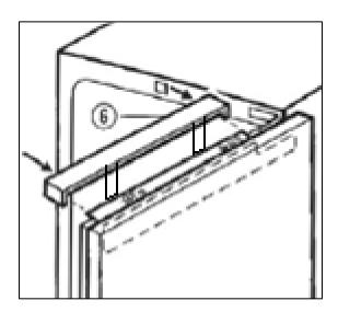
e) Insert the cover plate to the top of the appliance, this will just clip into place.
