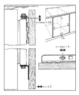
c) Use a screwdriver to adjust the gap on the lower section of the adjusting bolts. The gap should be set to approximately 9 mm (as shown in the above drawing).
