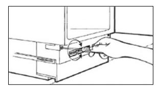
Remove the grid on the base of the appliance by unscrewing the screws on each side of the grid and then pull the grid towards you.
