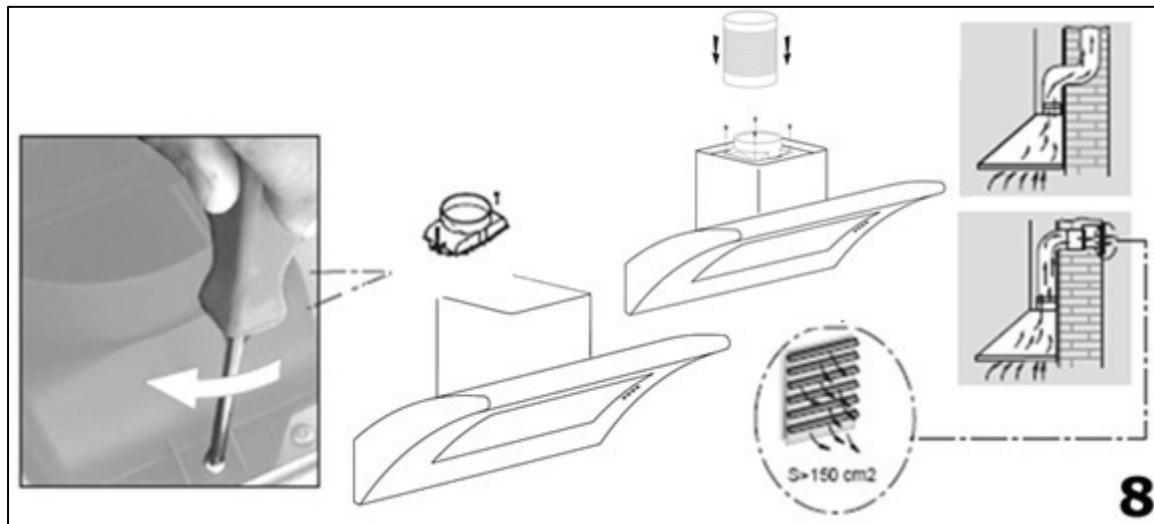
**8)** Connect the coupling to the top of the cooker hood, and then connect a 125 mm ducting hose to the coupling (please note that the ducting hose is not supplied with the appliance).
