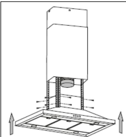
**6)** Lift the main body of the cooker hood onto the angle bar and then fix it into position using the 16 x M4 bolts.
