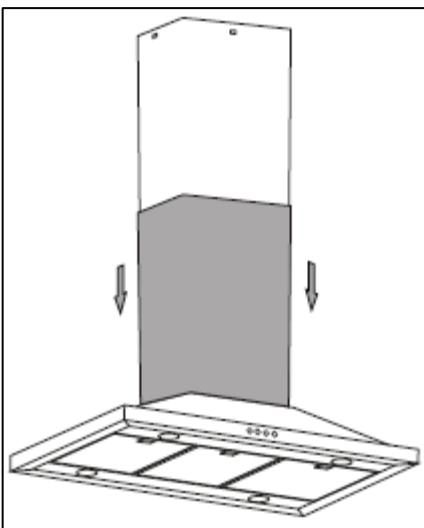
**8)** If you are going to be using the hood in extraction mode, you should fix the ducting hose to the spigot.
