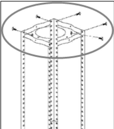
**2)** Fix the angle bars to the hanging plate, using the 8 x M4 nuts and bolts with metal washers.
