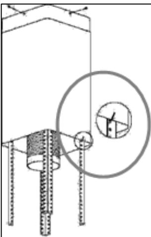
**4)** If your cooker hood is going to be used in extraction mode, then you should connect the ducting hose to the ceiling adaptor at this point.
