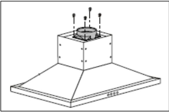
**5)** If you are going to be using the hood in extraction mode, you should fit the spigot for the duct hose onto the main body of the cooker hood, using the 4 x M4 bolts,
