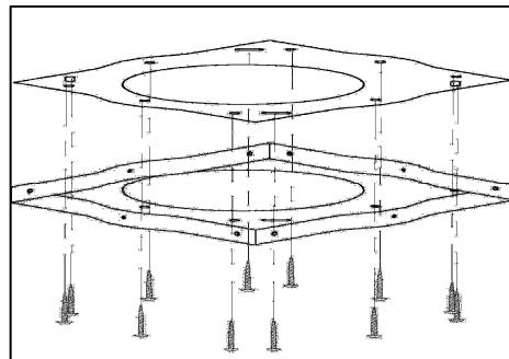
**1)** Position the hanging plate on the ceiling and then mark the position of the screw holes.
