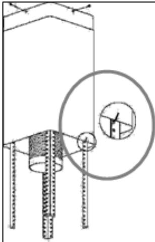
**5)** Fix the upper chimney section to the hanging plate, using the 4 x self tapping screws.
