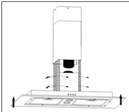
**7)** Lift the main body of the cooker hood onto the angle bar and then fix it into position using the 16 x M4 bolts.
