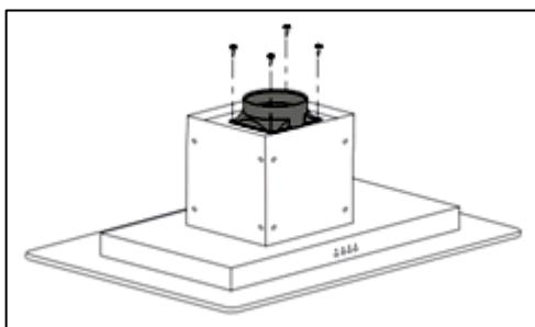
**6)** If you are going to be using the hood in extraction mode, you should fit the spigot for the duct hose onto the main body of the cooker hood, using the 4 x M4 bolts,
