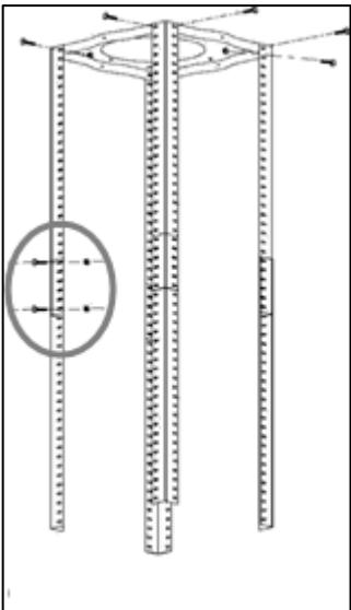
**3)** Extend the angle bars to the required height and then fix them in position using the 16 x M4 nuts and bolts with metal washers.
