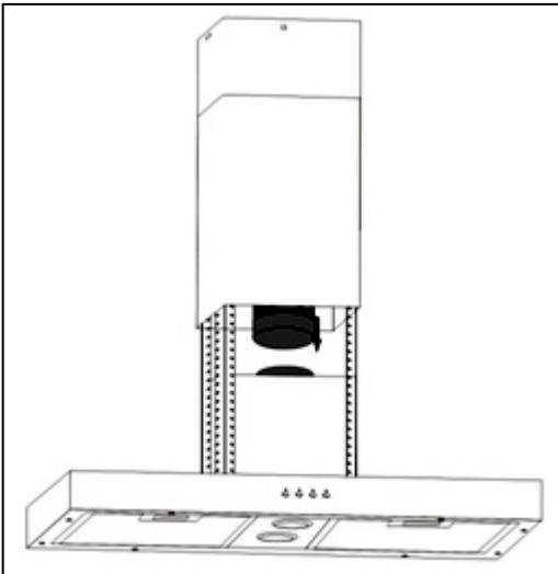
**8)** If you are going to be using the hood in extraction mode, you should fix the ducting hose to the spigot.
