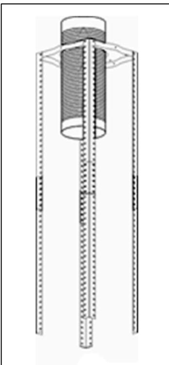
**4)** If your cooker hood is going to be used in extraction mode, then you should connect the ducting hose to the ceiling adaptor at this point.
