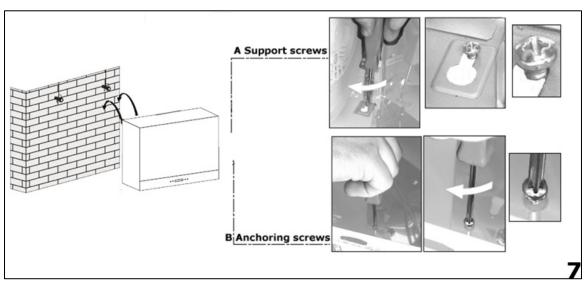
**7)** Fully tighten the support screws **(A)** and then screw the anchoring screws **(B)** through the relevant holes in the cooker hood. Fully tighten the anchoring screws into the wall.
