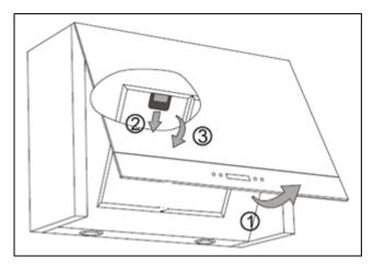
Lift up the cover that sits over the grease filter (as shown in the line drawing above).
