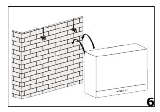
**6)** Hang the hood onto the support screws.
