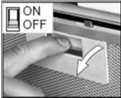
Remove the grease filter by pulling down on the handle and pulling it away from the cooker hood.
