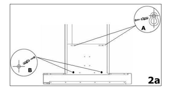
**2a)** The support screw holes are indicated by figure **A** in this drawing and the anchoring screw holes are indicated by figure **B**.
