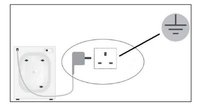
✓ IMPORTANT:The electrical socket must still be accessible once the appliance is installed.
