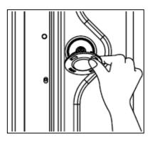
Cover the holes that you removed the transit bolts from, using the 4 transit covers supplied.
