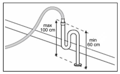
✓ Secure the drain hose, so that it cannot move whilst the washer dryer is in use.
