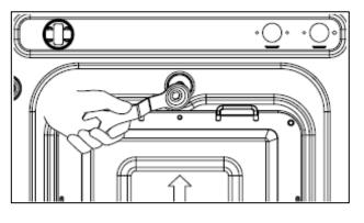
Using the spanner supplied, unscrew the 4 transit bolts.
