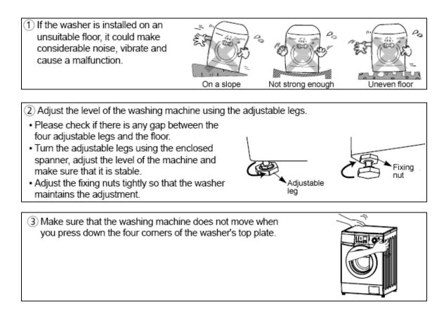
**IMPORTANT:** There should be no instability of the machine when the adjustable legs have been set to the correct level.
