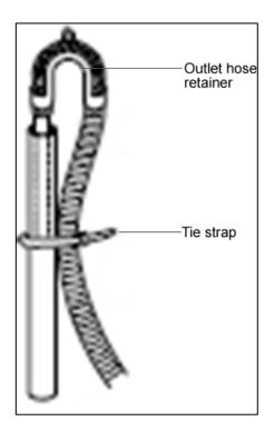
✓ Utilise the outlet hose retainer and tie strap to keep the outlet hose in position when the appliance is on a wash cycle.
