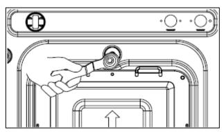
• Using the spanner supplied, unscrew the 4 transit bolts.
