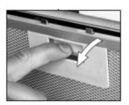
**1)** Remove the metal grease filters.
