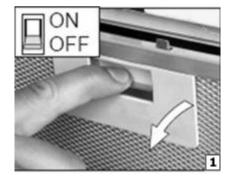
1) Remove the grease filters.
