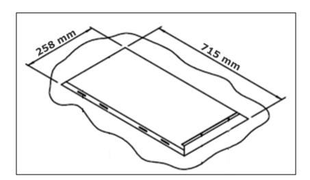
**2)** Create an opening in the underneath of the kitchen unit; the cutout must be of the dimensions shown in the drawing above.
