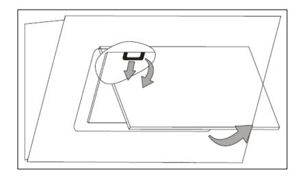
Open the cover screen at the front of the cooker hood, this will allow you to gain access to the grease filters.
