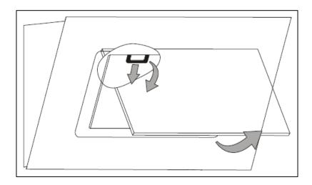
Open the cover screen at the front of the cooker hood, this will allow you to gain access to the grease filters.
