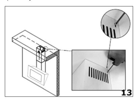
**13)** Lift chimney section **(D)** up to the ceiling and secure it to the L shaped bracket using the screws provided.
