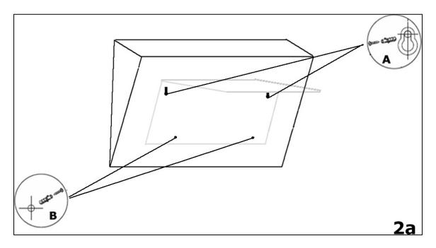
**2a)** The support screw holes are indicated by figure **A** in this drawing and the anchoring screw holes are indicated by figure **B**.
