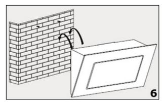
**6)** Hang the hood onto the support screws.
