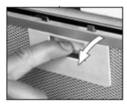
**1)** Open the cover screen and remove the metal grease filters.
