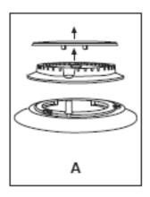
Remove the pan-stands, burners and flame spreaders (A).
