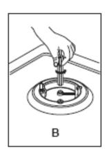
Unscrew the injector (B) and replace it with the stipulated injector for the new gas supply (see table below).
