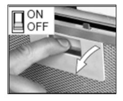
o Refit the grease filter.
