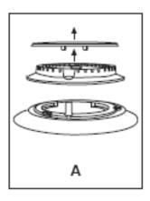
o Remove the pan-stands, burners and flame spreaders (A).
