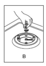
Unscrew the injector (B) and replace it with the stipulated injector for the new gas supply (see table on next page).
