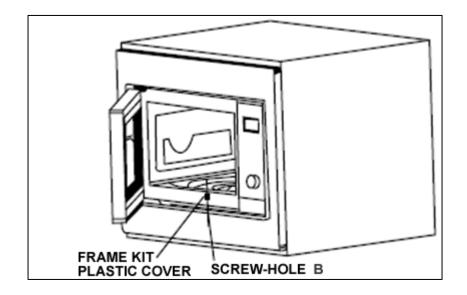
o Use the frame kit plastic cover and place it over screw-hole B.
