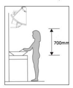
It must be positioned at least 700 mm above the hob underneath it. This measurement should be taken from the highest point on the hob, including the burners.
