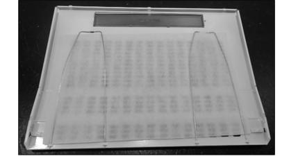
o Remove the metal wires which hold the synthetic filter in place.
