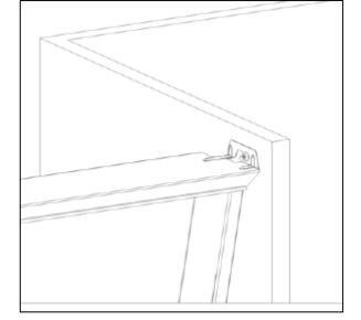
Hang the cooker hood onto the screws between the two cupboards.
