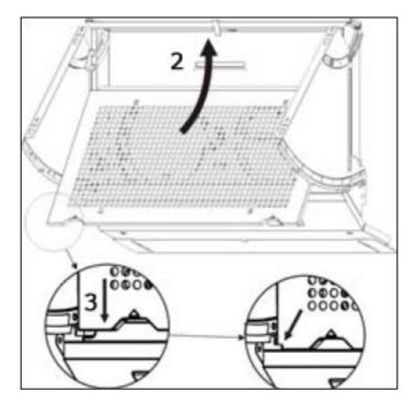
o Ensure the filter unclips from the hood, as shown in the diagram above (3), before you pull it away.
