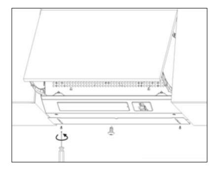
o Install the adjusting plate, in order to cover the gap between the wall and the bottom of the cooker hood, by screwing it into place.
