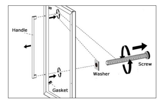
3) Install the handle on the outer right side of the door.
