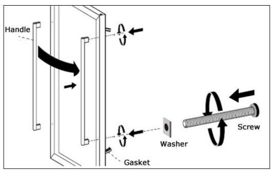
4) Install the 2 decorative screws in the holes on the left hand side of the outer door by following the instructions for removing the decorative screws in reverse (step 1).
