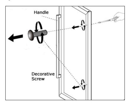
2) Remove the gasket on the left inner side of the door to expose the 2 handle screws. Unscrew them in an anti-clockwise direction with a cross screwdriver. Take out the screws and washers as well as the handle.
