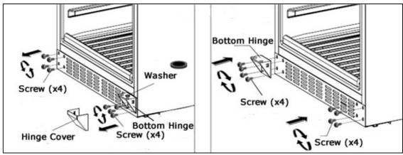
5) To reinstall the door on the opposite side, insert the door support rod into the bottom hinge through the washer and screw the upper hinge to the door. Finally, cover the hinge and hinge holes using the hinge covers.
