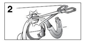
Carefully cut through the hose retaining clip at the rear of the appliance, taking care not to cut the hose (2).
