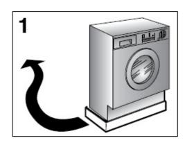
Remove the polystyrene base and place the machine near its permanent position (1).
