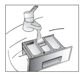
Pull the detergent drawer out as far as it will go and then remove the drawer by pulling firmly.
