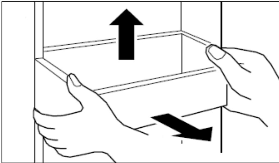
*It is possible to adjust the height of the general door racks and bottle racks in the doors.*
