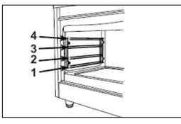
The oven walls of the two cavities are fitted with various guide bars on which you can place an oven shelf or a drip tray (see image below).
