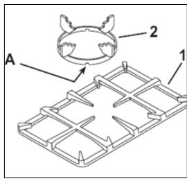
o The appliance is equipped with pan supports (1), on which the wok support (2) must be placed. To ensure stability, position the notch (A) of the wok support on the pan support fingers as indicated in the diagram above.
