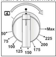
o Turn the dial clockwise to select a main oven temperature (50 °C -225 °C MAX).
