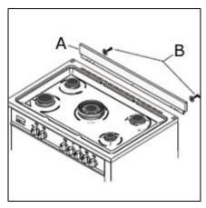
o Fix the back-guard into place by screwing the screws back into the hob with the back-guard placed in between.
