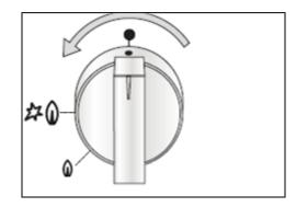
o Turn the relevant dial anticlockwise to select a power level for a chosen burner.
