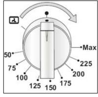
The oven temperature control knob should be turned clockwise to select the oven temperature.
