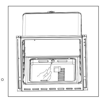
screw the injector and replace it with the required injector for the new gas supply according to the table below.
