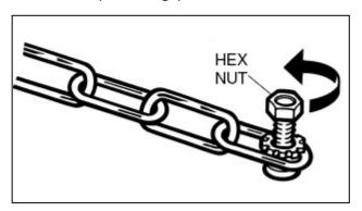
To fix the security chains to their anchor brackets: Unscrew the hex nut at the unattached end of the safety chain.
