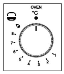
o To turn the main oven on, press and turn the control dial to the large flame position.
