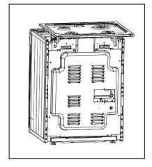
o When all the screws have been removed, slide the hob from the back to the front and lift it off the support brackets which hold the hob down at the front of the cooker.
