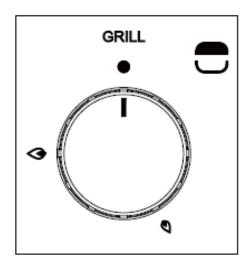
To turn the grill on press and turn the control dial to the large flame position.
