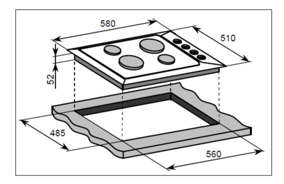
o Cut a hole in the worktop that corresponds with the drawing shown above.
