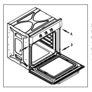
Ensure that the oven has been securely fixed into the housing unit. The fixing of the oven into the housing is made by using four screws. These should be screwed through the oven cabinet and into the housing
