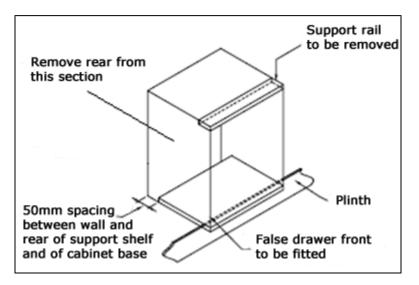
(Figure shows the ventilation and cut-out requirements for the installation of the appliance into a standard kitchen unit).
