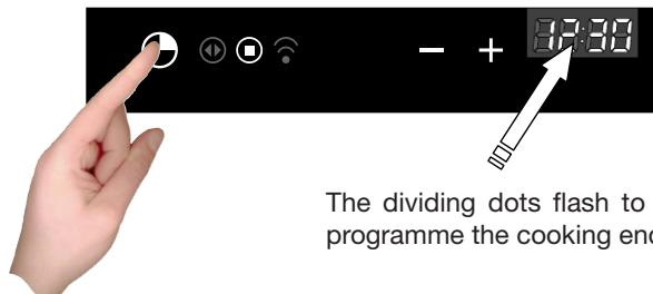
The dividing dots flash to indicate that it is possible to programme the cooking end time.
