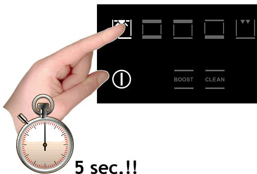
To disable the demo mode, touch the light symbol for five seconds: the controls will enter into standard operational mode and the oven is ready to be switched on.
