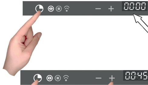
The dividing dots flash to indicate that it is possible to programme the cooking time
