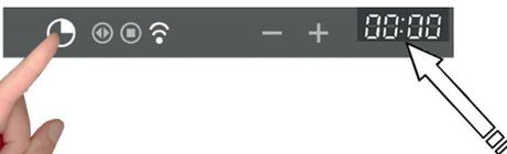
The dividing dots flash to indicate that it is possible to set the value.
