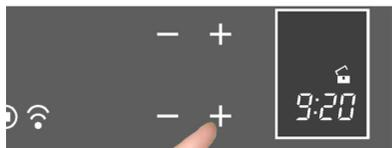
Adjusting the timer using the + and – keys: the separator dots flash at regular intervals (0.5 seconds) during the setting.
