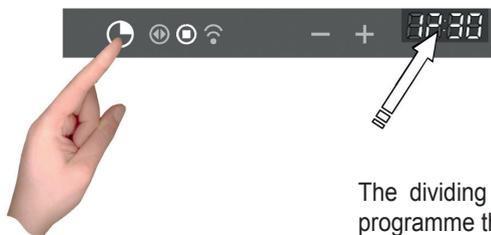
The dividing dots flash to indicate that it is possible to programme the cooking end time.
