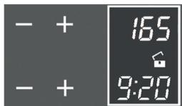
The OPEN padlock symbol means that the key function is not active.
