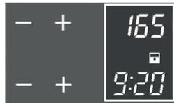
The CLOSED padlock symbol means that the key function is active.
