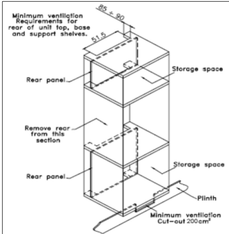
(Figure shows the ventilation and cut-out requirements for the installation of the appliance into a tall housing unit).
