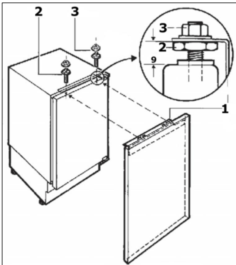
c) Hang the furniture door onto the appliance door, making sure that the brackets on the mounting bracket locate over the adjusting bolts.
