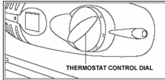
You switch on your appliance by connecting it to your mains supply and setting the thermostat. The thermostat control knob is located on the right hand side of the fridge.
