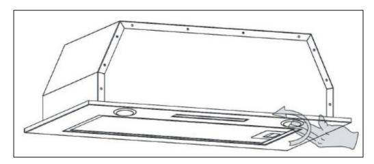
Press gently on the underside of the bulb that needs to be replaced and twist anticlockwise to release.
