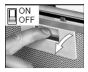
First remove the grease filters by pulling down on the handle and pulling them away from the cooker hood.
