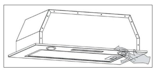
$\circ\,$  Press gently on the underside of the bulb that needs to be replaced and twist anticlockwise to release.
