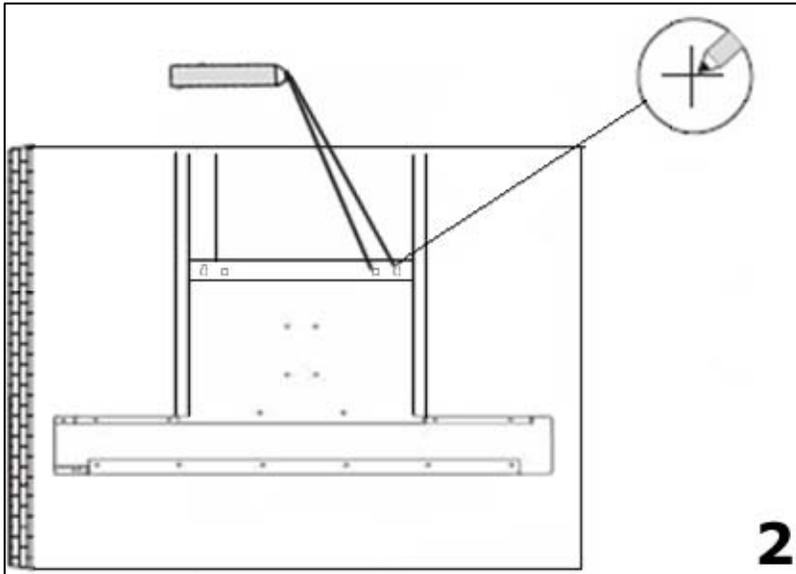
2) Position the hood against the wall that you are intending to install it on and mark the position of the support holes that are to be drilled (as shown in the figure opposite).
