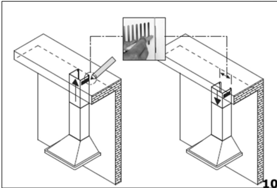
**10)** Lift chimney section **(D)** upwards until it reaches the ceiling. You must ensure that it is perpendicular to the hood.
