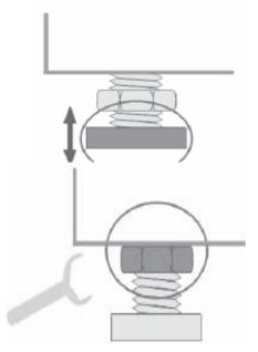
✓ Adjust the feet to level off the washing machine.
