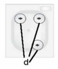
Place the supplied plastic stoppers into the holes on the back of the machine, which have been left by the removal of the transit bolts.
