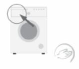
Replace the detergent drawer by slotting it into the slot and then pushing it back fully into position.
