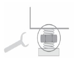
✓ Slacken off the lock nut on each of the washing machine feet using a spanner.
