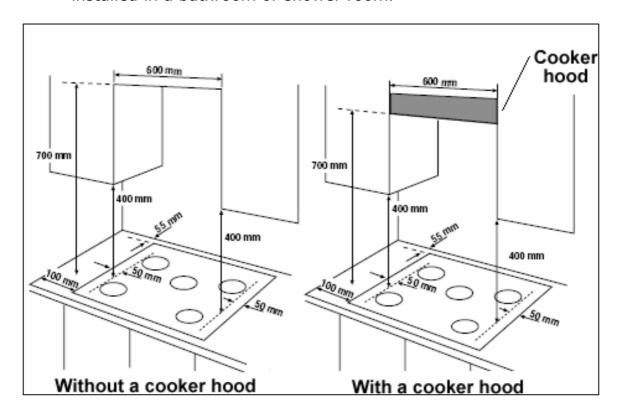
This appliance is classified as Class 3 and therefore is to be built into a kitchen unit (depending on size) or 600mm worktop, providing the following minimum distances are allowed:
