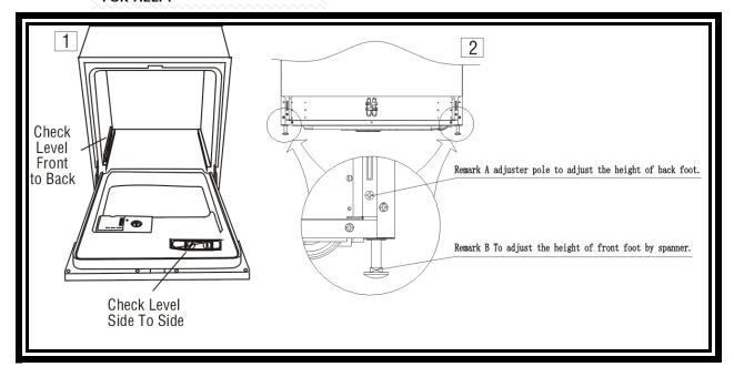
THE REAR FEET CAN BE ADJUSTED FROM THE FRONT OF THE DISHWASHER BY TURNING THE SCREWS ON THE LEFT AND RIGHT HAND SIDES OF THE CABINET. TO ADJUST THE FRONT FEET, USE A WRENCH / SPANNER AND TURN THE FRONT FEET UNTIL THE DISHWASHER IS LEVEL (PLEASE SEE 'REMARK B' IN THE ABOVE FIGURE).
