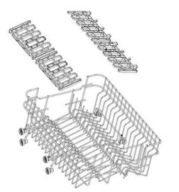
\*\*\*NOTE\*\*\*: THE UPPER RACK HAS SIDE FLAPS (PICTURED AT LEFT ABOVE BASKET). THERE ARE 4 (2 ON EACH SIDE). THESE CAN BE ADJUSTED INTO 2 POSITIONS = POSITION 1 (HIGH) AND POSITION 2 (LOW).
