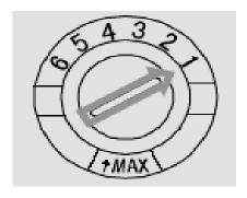
The rinse aid dispenser has six settings. ALWAYS START WITH THE DISPENSER SET ON "1". IF SPOTS & POOR DRYING ARE A PROBLEM, INCREASE THE AMOUNT OF RINSE AID DISPENSED BY REMOVING THE DISPENSER LID AND ROTATING THE DIAL TO "2". IF THE DISHES ARE STILL NOT DRYING PROPERLY OR ARE SPOTTED, ADJUST THE DIAL TO THE NEXT HIGHER NUMBER UNTIL YOUR DISHES ARE SPOT-FREE.
