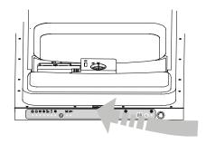
TO CLEAN THE EDGE AROUND THE DOOR, ONLY EVER USE A SOFT WARM, DAMP RAG. DO NOT USE A SPRAY CLEANER HERE OR WHEN CLEANING THE DOOR PANEL AS THIS MAY HARM THE DOOR LOCK AND ELECTRICAL PARTS.
